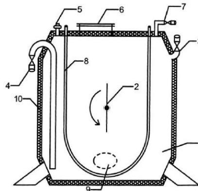
**Fig. 1.** Bioreactor scheme: 1 – reservoir; 2 – means of mixing; 3 – download branch pipe; 4 – discharge branch pipe; 5 – valve; 6 – hatch; 7 – biogas exit pipe; 8 – heating system; 9 – hatch; 10 – a layer of thermal insulation.
