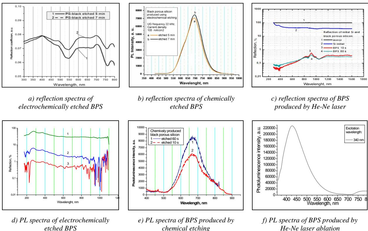
Fig. 4. The spectra of reflection and photoluminescence of black porous silicon layers
