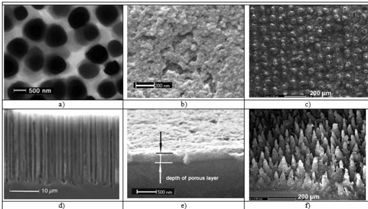
Figure 3. The SEM view from the top and from the side of black porous silicon, produced using electrochemical etching (a, d), chemical etching (b, e) and ablation by laser (c, f) method
