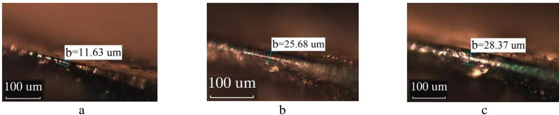
4 pic. Optical images of the cutting edge width b of WC+TiCN cutter: a - L = 130 m; b - L = 11130 m; c - L = 26130 . (150 x).
