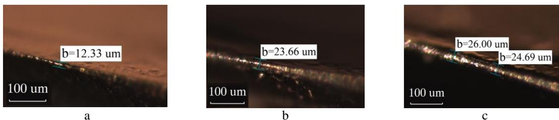
6 pic. Optical images of the cutting edge width  $b$  of WC+DLC cutter: a -  $L = 130$  m; b -  $L = 11130$  m; c -  $L = 26130$  .
