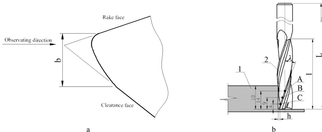
Fig. 1. Measurement schemes of the helical cutting edge width  $b$ : a – cross-section of the cutting edge; b – scheme of measurement points of the cutting edge width  $b$ ; 1 – sample; 2 – router cutter; A, B and C – measurement points;  $h$  – depth of milling;  $\lambda$  – inclination angle
