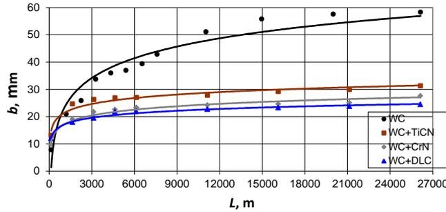
Fig. 2. Influence of the cutting path L on the cutting edge width b.
