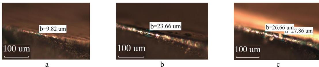
5 pic. Optical images of the cutting edge width  $b$  of WC+CrN cutter: a -  $L = 130$  m; b -  $L = 11130$  m; c -  $L = 26130$  .
