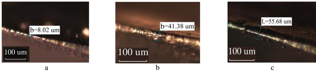
3 pic. Optical images of the cutting edge width b of uncoated WC cutter: a - L = 130 m; b - L = 11024 m; c - L = 26130 . (150 x).
