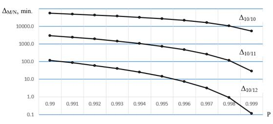
Figure 4. The dependence of non-working time  $\Delta_{M/N}$  on P values and the number of reserve computers (N-M)
