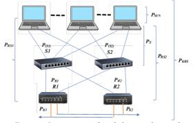
Figure 3. Reservations of workplaces and network equipment
