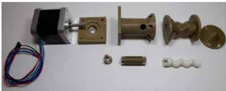
3. Figure. Parts of progressive cavity pump's extruder.
