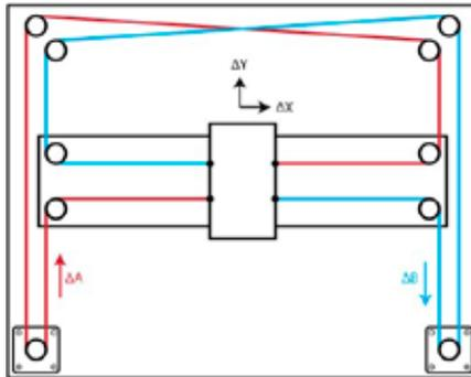
1. Figure. CoreXY principle.[1]
