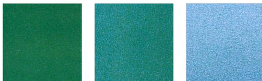
*Figure 1. The change in the appearance of green colour enhanced with pearlescent pigment (Iridodin® 221 Rutil Feinblau) with the change of the illumination angle (angle was increased in the steps of 30°)*
