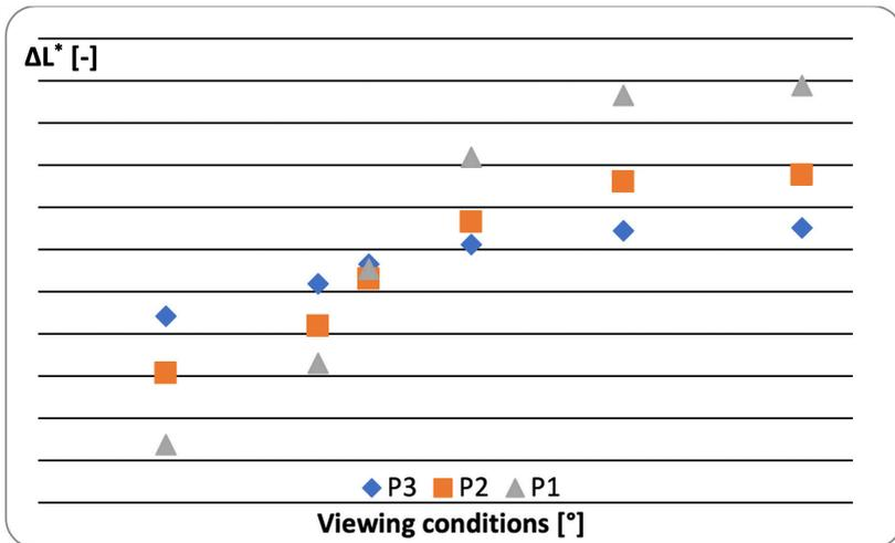
Fig. 2.  $\Delta L^*$  parameter changes of blue metallic ink observed under different angle viewing conditions in reference to the thickest ink film amount applied on the gloss coated paper, P1 –  $0.05 \text{ cm}^3$ , P2 –  $0.15 \text{ cm}^3$ , P3 –  $0.3 \text{ cm}^3$
