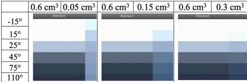
Fig. 1. Changes in colour of blue metallic ink on gloss coated paper due to different viewing conditions ( $-15^\circ$ ,  $15^\circ$ ,  $25^\circ$ ,  $45^\circ$ ,  $75^\circ$ ,  $110^\circ$ ) and different ink film thicknesses.
