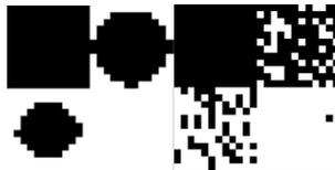
*Fig 2. Raster dots with 0%, 20%, 50% and 100% dot area rate after printing
