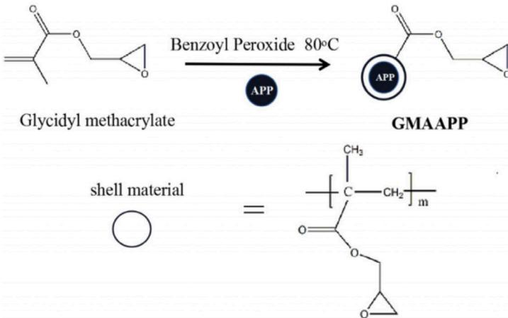
Fig 1. The encapsulation process of ammonium polyphosphate
