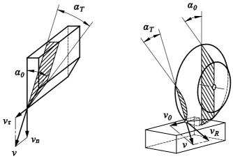
a) Flat cutter b) Circular cutter Fig. 3. The scheme of a knife sharpening edge transformation.
