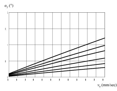
Fig. 6. Kinematic reduction of sharpening edge angle  $a_T$  by different feed rates  $v_{qr}$  Counter-synchronous cutting. n=3000rpm.
