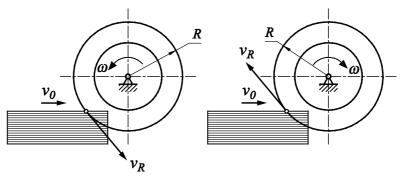
a) Synchronous cutting b) Anti-synchronous cutting Fig.1. The schemes of cutting processes with circular cutters
