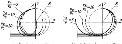
a) Synchronous cutting b) Anti-synchronous cutting Fig. 2. Movement trajectories of the point at the edge of cutter
