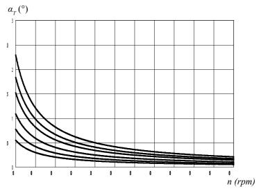
Fig. 5. Kinematic reduction of sharpening edge angle  $a_T$  by different rotation speeds n. Counter-synchronous cutting.  $v_0=1000$  mm/sec.
