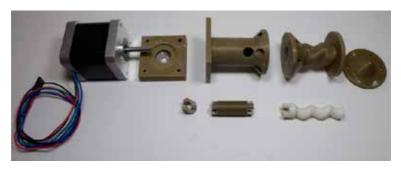
3. Figure. Parts of progressive cavity pump's extruder.
