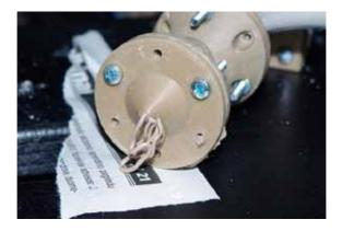
5. Figure. Clay's flow through nozzle
