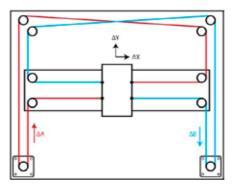
1. Figure. CoreXY principle.[1]
