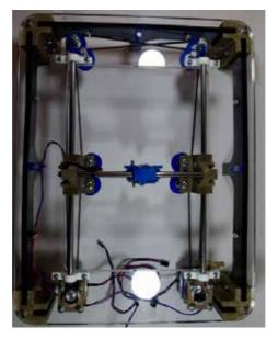
2. Figure. Built CoreXY board.
