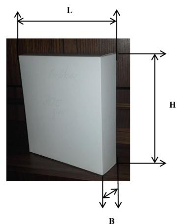
Figure 1 Specimens (packages): box size (H=200 mm, L=170 mm, B=50 mm)
