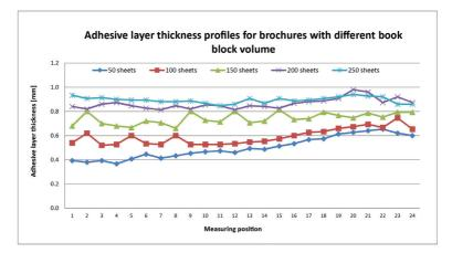
Figure 2 – Adhesive layer thickness profiles for brochures with different book block volume
