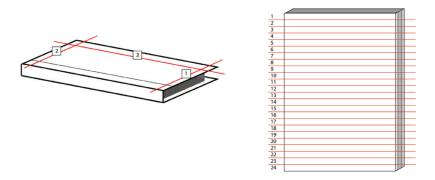
a) b) Figure 1 – Cutting sequences for book block 3-side trimming (a) and measurement segments preparing (b)
