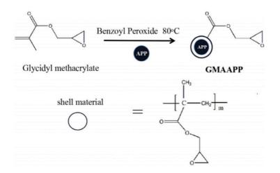
Fig 1. The encapsulation process of ammonium polyphosphate
