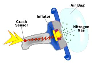
**Fig. 4.** The airbag and inflation system stored in the steering wheel
