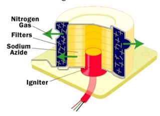
**Fig 3.** The inflation system with a solid propellant and an igniter
