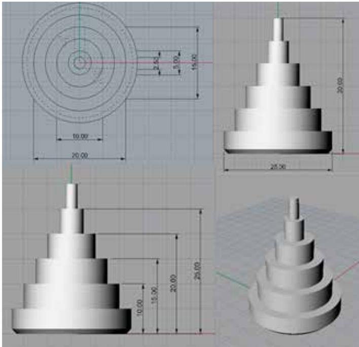
*Figure 2 Digital 3D model of printed objects*
