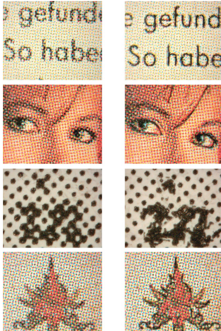
Figure 4. Fragmentary microphotographs of 4-color half-tone prints produced at 175 Lpi and screening factor of 2.0 with the use of Scitex Class Screening (left) and HDHP (right)
