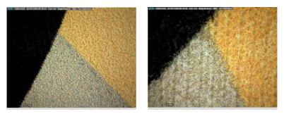
Fig. 4. Thermal transfer printing (the first) and direct printing (the second), the sample  $(50 \times)$
