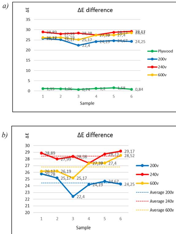
Fig 3. Colour difference  $\Delta E$  on glued plywood exposed to radiation:
