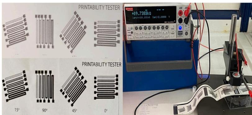
*Figure 2. Flexography printed patterns, on the same paper; using the G/MWNT-*f*-OH hybrid with total solids carbon/resin ratio (left and up) 55/45 (left and down) 70/30. (Right) Measurement of the  $V/I$  of the printed pattern (with total solids carbon/resin ratio 70/30)*
