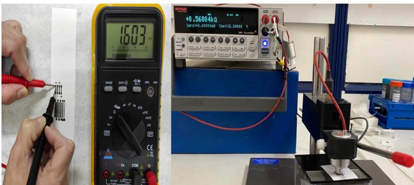
Figure 5. Various V/I measurements of the screen printed pattern
