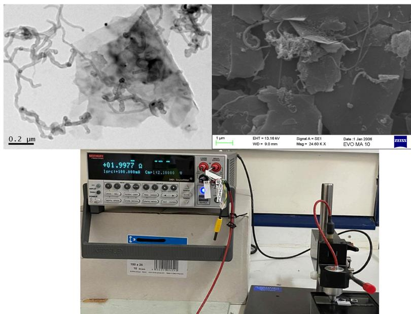
Figure 1. Representative TEM (Up and left) and SEM (Up and right) images of the carbon hybrid (Down) Measurement of the V/I of the hybrid
