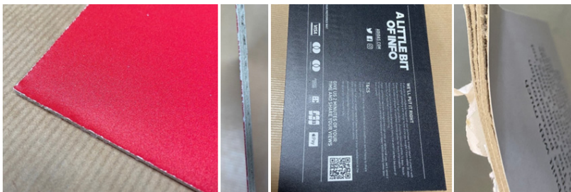
Fig.1. Examples of poor die-cutting, delamination, and poor water resistance of Katz Displayboard
