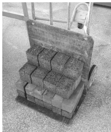
Fig. 2. Expanded concrete blocks made for the study
