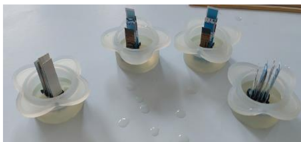
Fig. 3. Samples after pouring the epoxy resin
